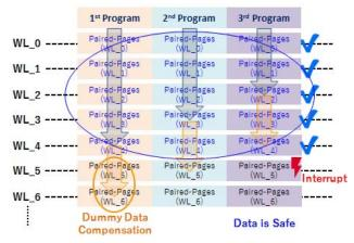
Figure 3-14: Dummy Data Compensation
