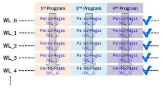
Figure 3-11: Programming Operation of TLC Flash
