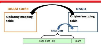
Figure 3-8: Rebuilding Metadata Mapping Table
